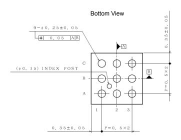
9pin WL-CSP (VCSP50L1) [  $1.7 \times 1.7 \times 0.55$ mm Max, 0.5mm Pitch ] (Unit : mm)
