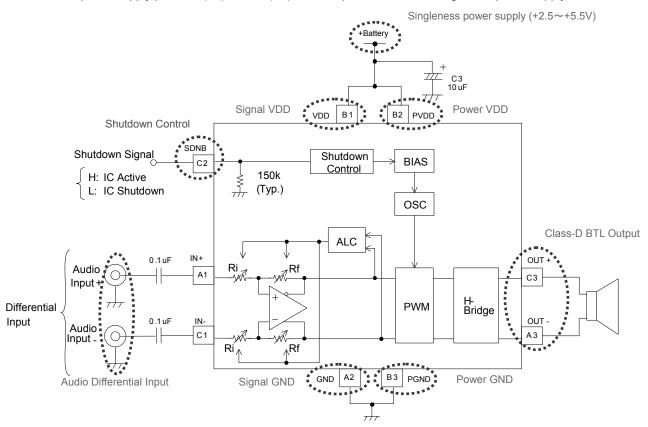
Fig1. Differential Input (With Input Coupling Capacitor)
