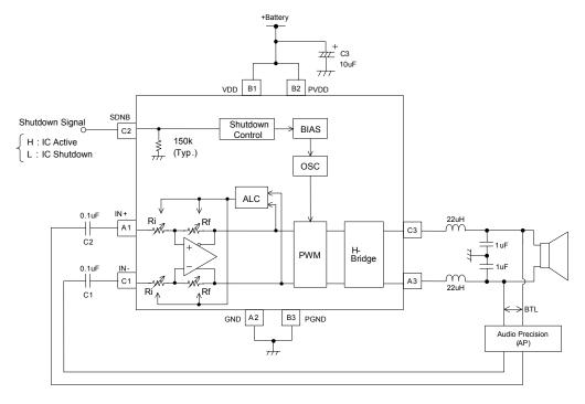
Audio characteristics can be measured to insert LC filter between output pin and speaker load, if you don't have measurement equipment for switching amplifier, like AUX-0025, Audio Precision.
