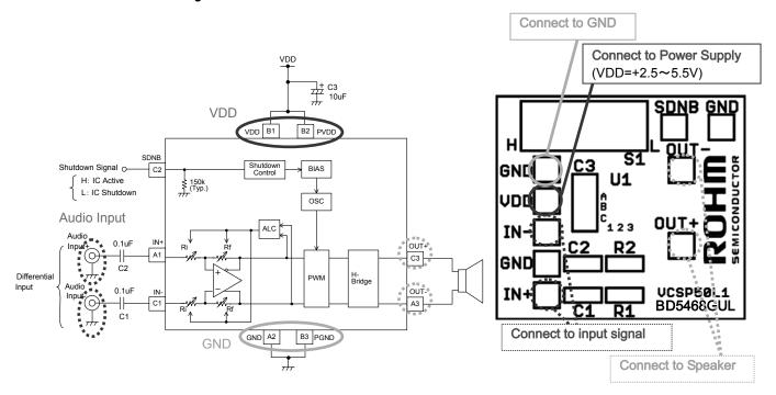
\*\*Power Supply terminals VDD(B1), PVDD(B2) are SHORT in the board pattern and use a single power.
