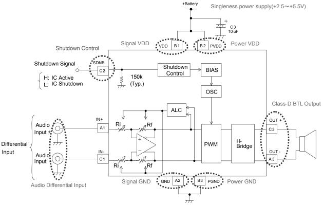
Fig2. Differential Input (Without Input Coupling Capacitor)
