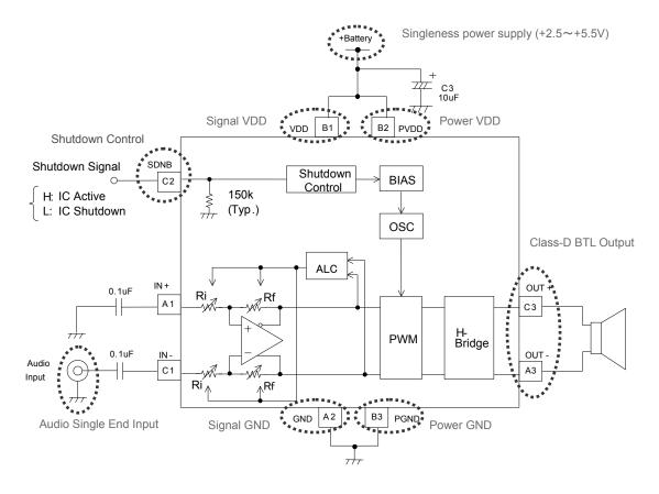
Fig4. Single end input (during IN- Input)
