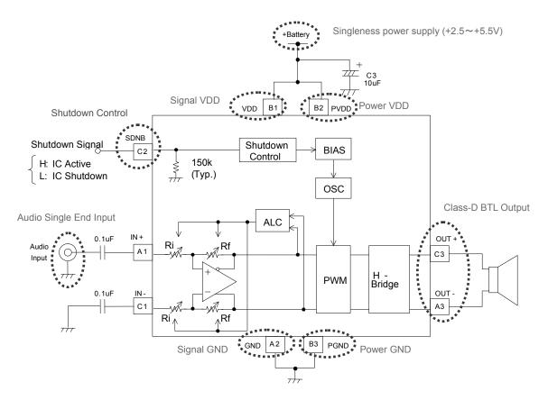
Fig3. Single end input (during IN+ input)
